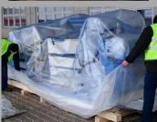
When metals are wrapped or packaged in this VCI film, the VCI chemicals form a protective molecular layer on the surface of the metal. This protective layer serves as a barrier, preventing moisture, salt, dirt, oxygen, and other corrosion-causing materials from depositing directly on the metal and causing rust and corrosion. When the part is unwrapped, the VCI will safely dissipate. No further cleaning is required.
