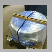
Packaging personnel should always wear gloves while handling metal parts. Parts should be clean and free of fingerprints before wrapping. Package clean products as quickly as possible. Place the part no more than 12" (30 cm) from the Premium Metal-Guard Stretch film. Stretch film can be used over Daubert Cromwell VCI papers for additional protection when needed.
