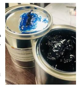
Exposed metal that is protected with Nox-Rust 1150 can be packaged immediately without waiting, which improves the speed of handling
