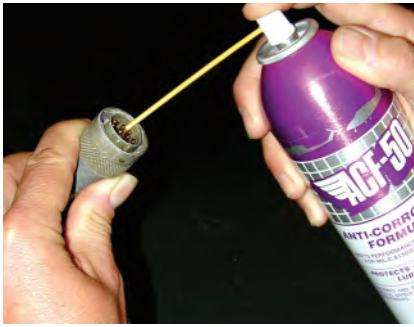
ACF-50 (Anti-Corrosion Formula) lubricant 'creeps' into tight seams, lap joints and around rivet heads to displace moisture and corrosive fluids such as orange juice, Coke and salt water. Learchem image.
